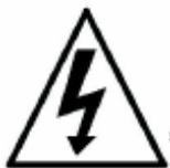
This symbol is intended to alert the user of the presence of non insulated "dangerous voltage" within the products enclosure that may be of sufficient magnitude to constitute a risk of electric shock to persons.
